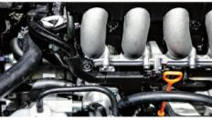
**11.** To replace metal, engine parts can be engineered from Rilsan<sup>®</sup> HT, a polyamide that withstands high temperatures and reduces engine weight. It is:
