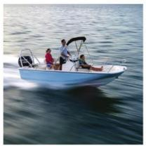
This pleasure boat has structural parts and a hull made from a fiberglass and Elium® resin composite. Thanks to Elium®'s thermoplastic nature (the resin can be heated and recovered), these parts are fully recyclable at end of life, and can be
